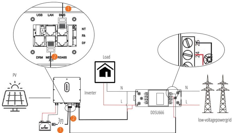
Note: ① is only for lithium battery. Meter is optional.
