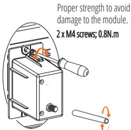
Proper strength to avoid damage to the module.
