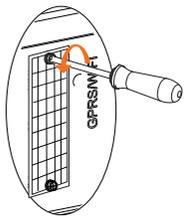
Loosen two screws and move the cover.
